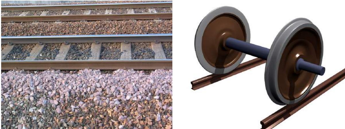
Figure 4.10: The ballast on a railway track and the axle of a train bogie
