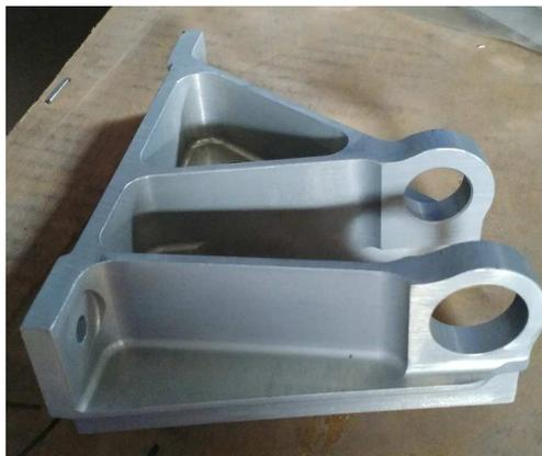
Figure 7: The regular aluminium bracket of case study 2
