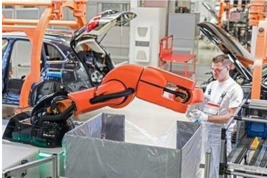
Fig. 2. Collaborative actor in car manufacturing: human working hand-in-hand with robot [11]
